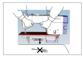
To prevent possible accidents caused by the full of the sewing machine, perform the work by two persons or more when the machine is moved.
