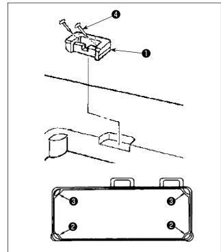
3) Place rubber cushions 2 and 3 at four corners of the table groove. Secure each of them with nail 4 (one piece).
