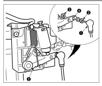
Fix connecting rod ① to installing hole ④ of pedal lever ② with nut ③ .
