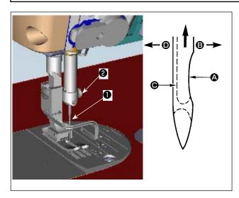
Use the specified needle for the machine. Use the proper needle in accordance with the thickness of thread used and the kinds of the materials.
