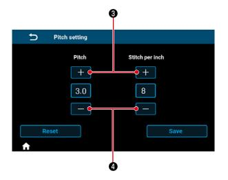
The stitch length is set to the value that corresponds to the number of stitches per inch by inputting the number of stitches per inch with the + and - buttons.
