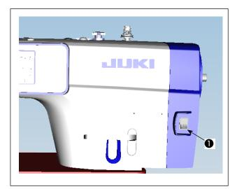
Reverse feed stitching at the beginning of sewing, reverse feed stitching at the end of sewing and various sewing patterns can be set on built-in panel of the machine head.
