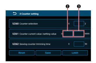
Set the counter set value in ③ of U261 on the counter setting screen. The counter setting screen is displayed when the current value ④ on the counter reaches the set value when the sewing machine carries out sewing while the sewing screen is displayed.
