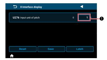
The stitch length can be set using the number of stitches per inch by setting "U276 Input unit of pitch" to ①.
