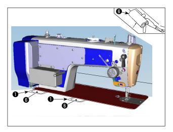
5) Attach supplied under-cover (5) to the underside of the table with six wood screws.(The notch should face the worker.)
