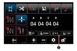
In the case the function of setting the number of stitches per inch is enabled, the screen for setting the number of stitches per inch is displayed by pressing the stitch length button \$\$\frac{1}{2}\$.
