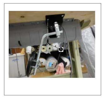
Install the knee lifter (asm.) on the underside of the table near the notch on the under-cover with four supplied mounting screws 1.
