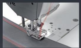
3-needle operations with 4,8 mm needle gauge, e.g. leather or airbag applications
