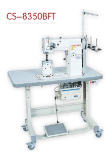
Double Needle, Unison Feed, Postbed Sewing Machine, (With automatic undertrimming & backtacking & presser foot lifting) (Large hook)
