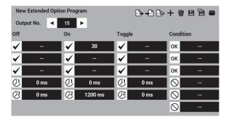
3. Referring to the table of condition numbers of the extended option output (refer to page 86), set the output condition for No. 16 to "condition No. 98 (when No. 15 is turned on)". Set Timer 1 to 0.5 sec. (500 ms) and Timer 2 to 0.7 sec. (700 ms).
