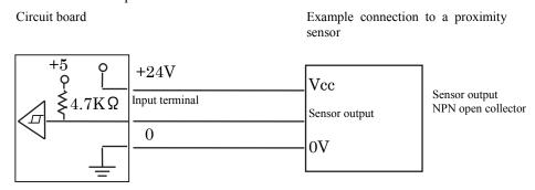
• In addition to using a contact switch or a 24 V sensor, use relays to isolate inputs.
