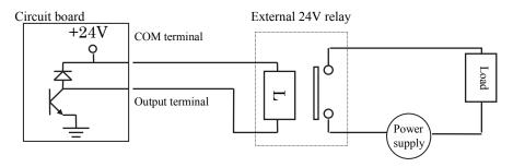
Fuses are not incorporated into the output circuit. To prevent the circuit from being damaged if the output short-circuits, it is recommended that you mount an external fuse for each circuit.
