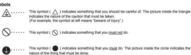
(For example, the symbol at left means "you must make the ground connection".)
