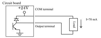
It is assumed that an optionally available air valve is used. In addition to a 24 V air valve, use a 24 VDC relay.
