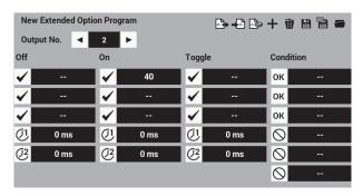
4. Referring to the "External input of the extended option" table of condition numbers (refer to page 86), set the output off condition for No. 2 to "off when condition No. 41 (input 1 off) is established". Enter into the setting screen as follows.
