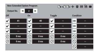
5. Referring to the "External input of the extended option" table of condition numbers (refer to page 86), set the enabling condition for No. 2 to "Enable ok setting when condition No. 42 (input 2 on) is established". Set "Disable when condition No. 43 (input 2 off) is established".
