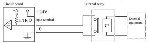
• Use relays for an electronic circuit with a min. application load of 5 V and 1 mA or less.
