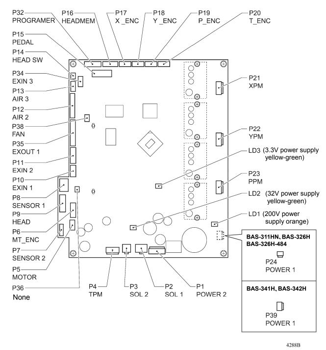
Connector layout of the main circuit board (BAS-360H, BAS-365H, BAS-370H, BAS-375H)
