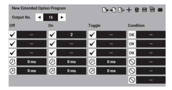
3. Referring to the "Mode for operating the sewing machine" table of condition numbers (refer to page 85), set to "off when condition No. 3 (before sewing start) is established".
