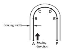
Be sure to press (J) twice to make a split at a point B or E where the line changes to the curve.
