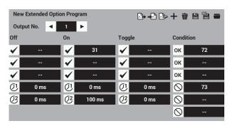
3. Referring to the "External input of the extended option" table of condition numbers (refer to page 86), set the enabling condition for No. 2 to "Enable setting when condition No. 40 (input 1 on) is established". Enter into the setting screen as follows.
