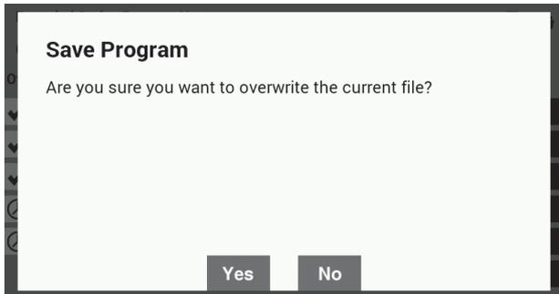
\* The save screen is not displayed when "Single SEQ file mode" in "Programmer" is set to "ON". Furthermore, during single SEQ file mode, a confirmation screen is displayed asking if you would like to apply the extended option output settings to the sewing machine immediately after saving them.
