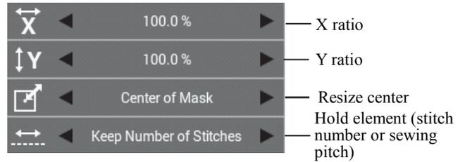
\* Resize center ... Origin, Center of Mask, Mask top edge, Mask bottom edge, Mask top-left, Mask bottom-left, Mask top-right, Mask bottom-right, Specified point
