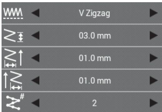
5. Set the running pitch and zigzag width for V-type zigzag stitches.
