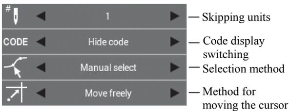
\* If the method for moving the cursor is set to "Move freely", the cursor can be moved to any desired position.
