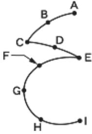
Be sure to press
