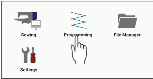
\* When "Starting extended option editing directly" in "Programmer" is set to "ON", touch
