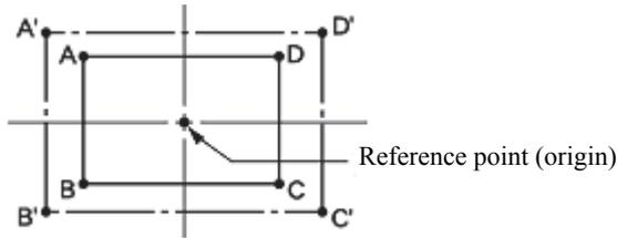
The reference point for resizing patterns is the center point for enlarging or reducing the pattern size.
