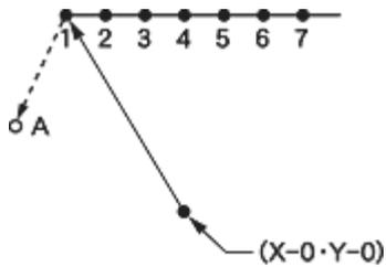
\* The escape point is a provisional point provided to preventing the work clamp from interfering with the needle or the presser foot when the work clamp is lifted at the start point.
