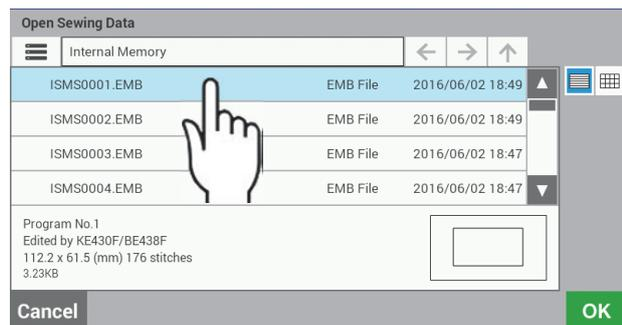
4. The details of the file which have been loaded will appear in the programming screen.
