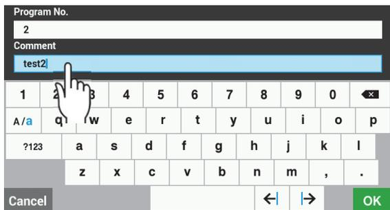
4. When you touch **OK** on the numeric keypad screen or the keyboard screen, the file will be saved in the panel internal memory and the display will return to the programming screen. Touch **Cancel** to return to the programming screen without saving the file.
