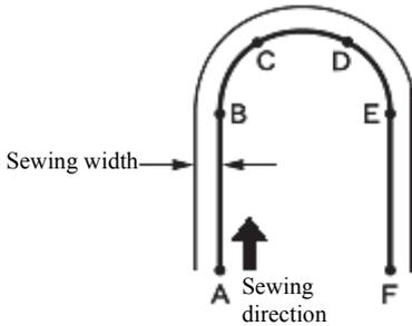
Be sure to press
