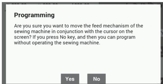
Furthermore, if you press **No** at the above screen, the model selection screen (shown below) will be displayed, so select the applicable model and then touch **OK**. At this time, you can create programs without operating the sewing machine.
