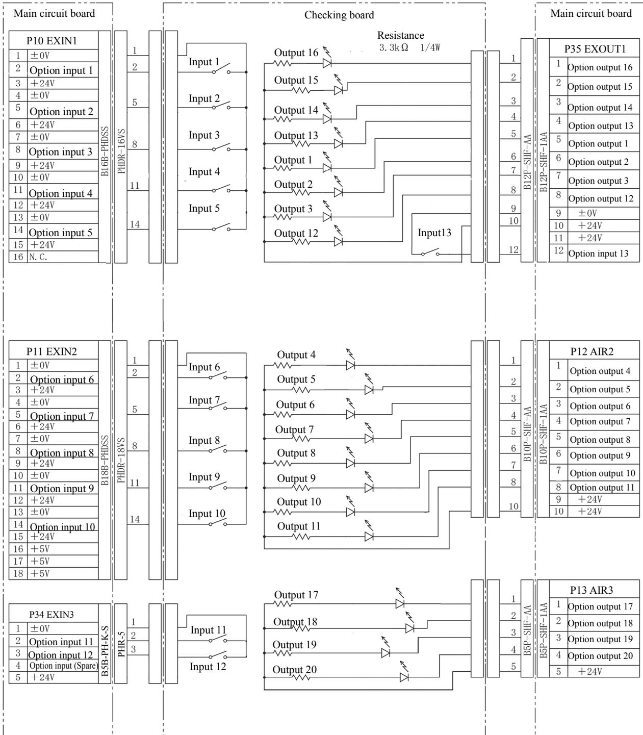
Option input 14 is a connector shared with the home position sensor signal. It is not used on the checking board.
