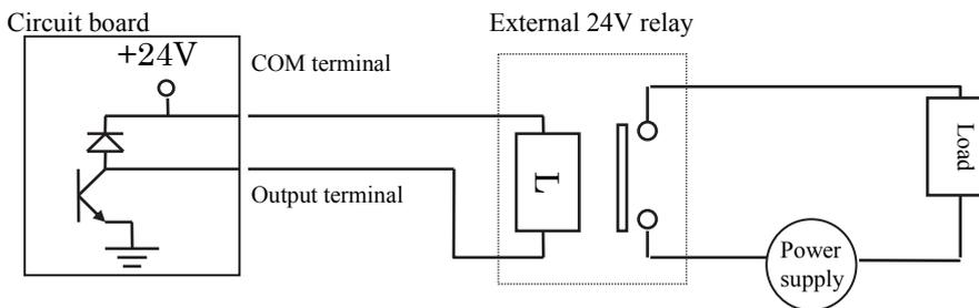
Fuses are not incorporated into the output circuit. To prevent the circuit from being damaged if the output short-circuits, it is recommended that you mount an external fuse for each circuit.
