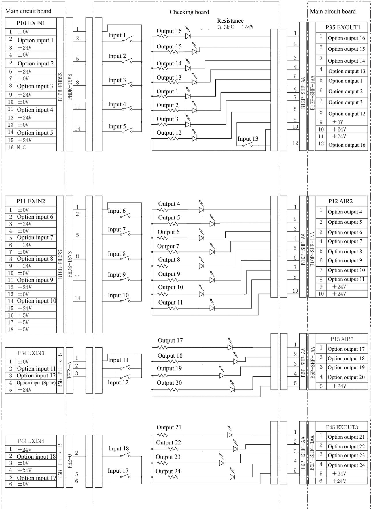
Option input 14 is a connector shared with the home position sensor signal. It is not used on the
