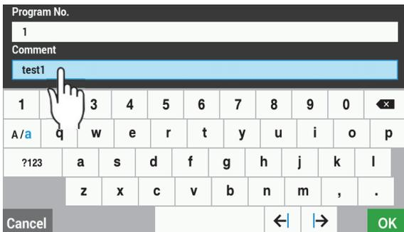
4. When you touch **OK** on the numeric keypad screen or the keyboard screen, the file will be saved in the panel internal memory and the display will return to the programming screen. Touch **Cancel** to return to the programming screen without saving the file.
