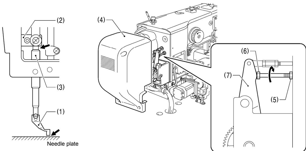
1. With the intermittent presser foot (1) lowered, turn the pulley in the direction of the arrow to move the intermittent presser foot (1) to its lowest position.
