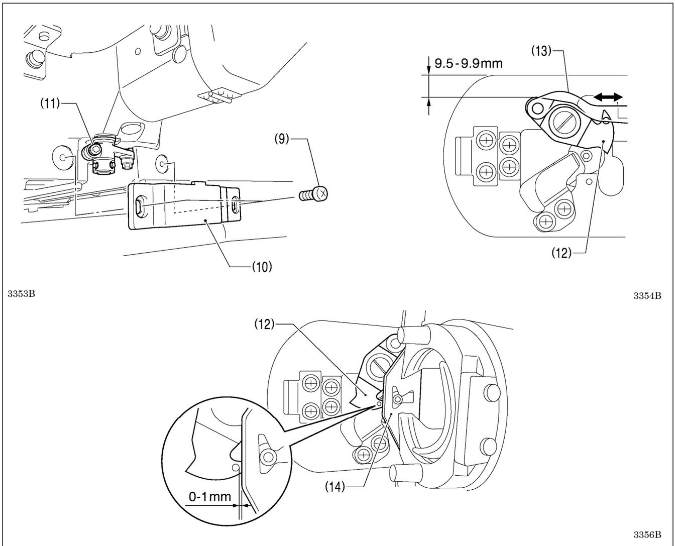
7. Loosen the two screws (9), and then remove the cover (10).
