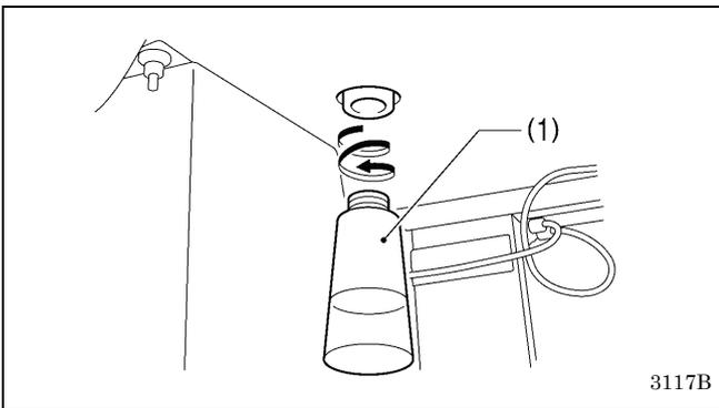
1. Remove and empty the waste oil tank (1) whenever it is full.
