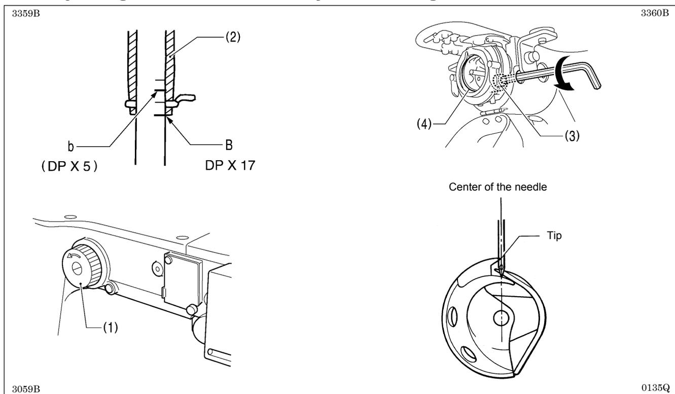
1. Turn the pulley (1) in the direction of the arrow to raise the needle bar from the lowest position until the lowest reference line on the needle bar (reference line B) is aligned with the lower edge of the needle bar bush (2).
