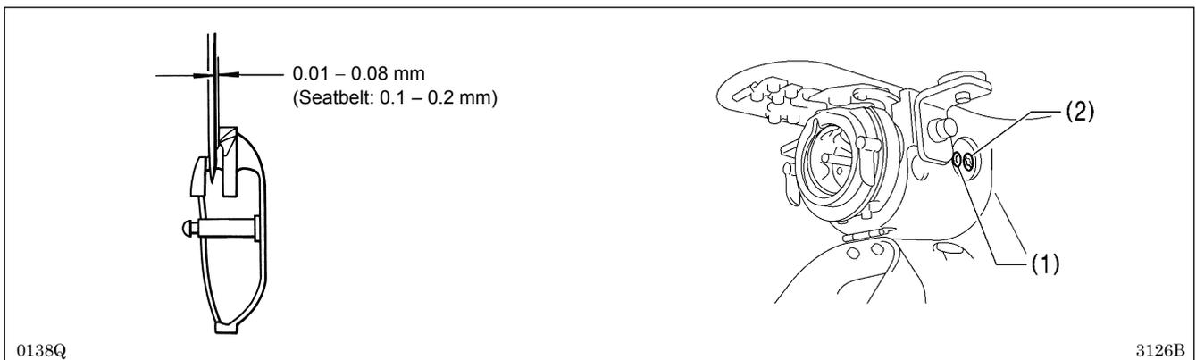
Turn the pulley in the direction of the arrow to align the tip of the rotary hook with the center of the needle, and then loosen the set screw (1) and turn the eccentric shaft (2) to adjust so that the clearance between the needle and the tip of the rotary hook is 0.01 to 0.08 mm.
