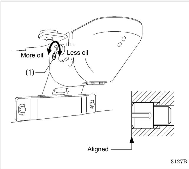
The optimum position is when the head of the set screw (1) is aligned with the edge of the bed. The rotary hook lubrication amount can be adjusted within three turns to the right from that position.
