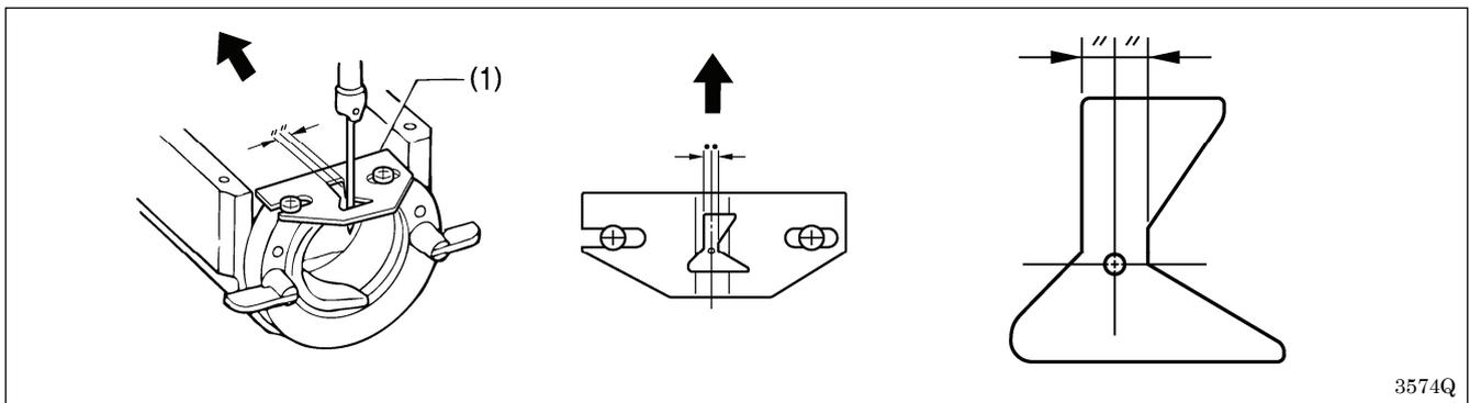
Install the shuttle race thread guide (1) by pushing it in the direction of the arrow so that the needle groove is aligned with the center of the needle plate hole.
