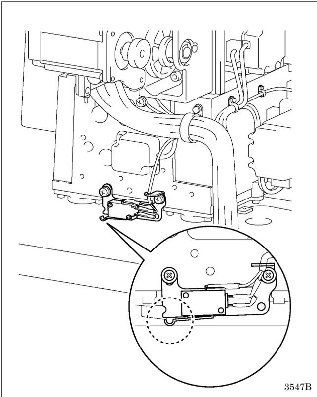
Check that the machine head switch is turned on as shown in the illustration.
