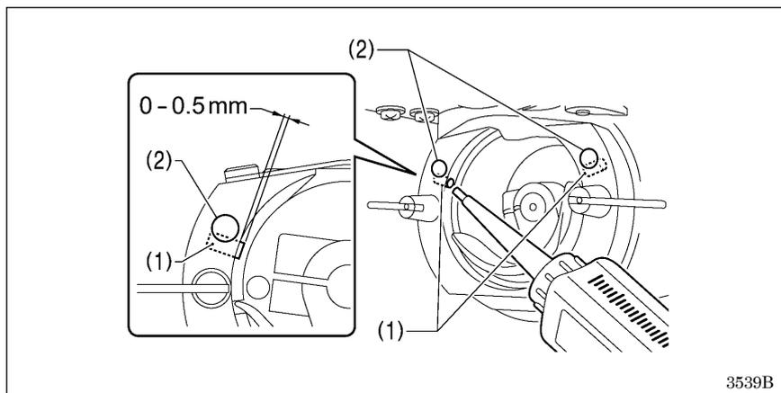
3. Pour oil in through the two holes of the shuttle race base assembly so that the felt (1) is lightly moistened.
