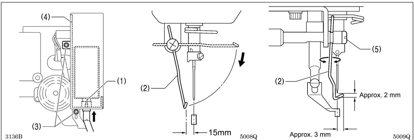
1. Loosen the two screws (3) and shift the entire solenoid setting plate (4) up or down to adjust so that the thread wiper (2) is 15 mm in front of the needle center when the plunger (1) of the thread wiper solenoid is driven to the full stroke.
