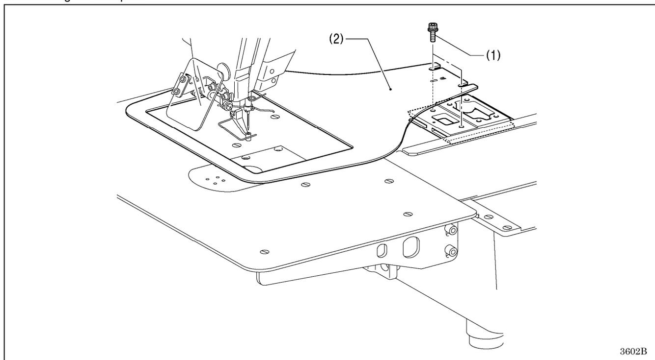
Loosen the two bolts (1), and then remove the feed plate (2).
