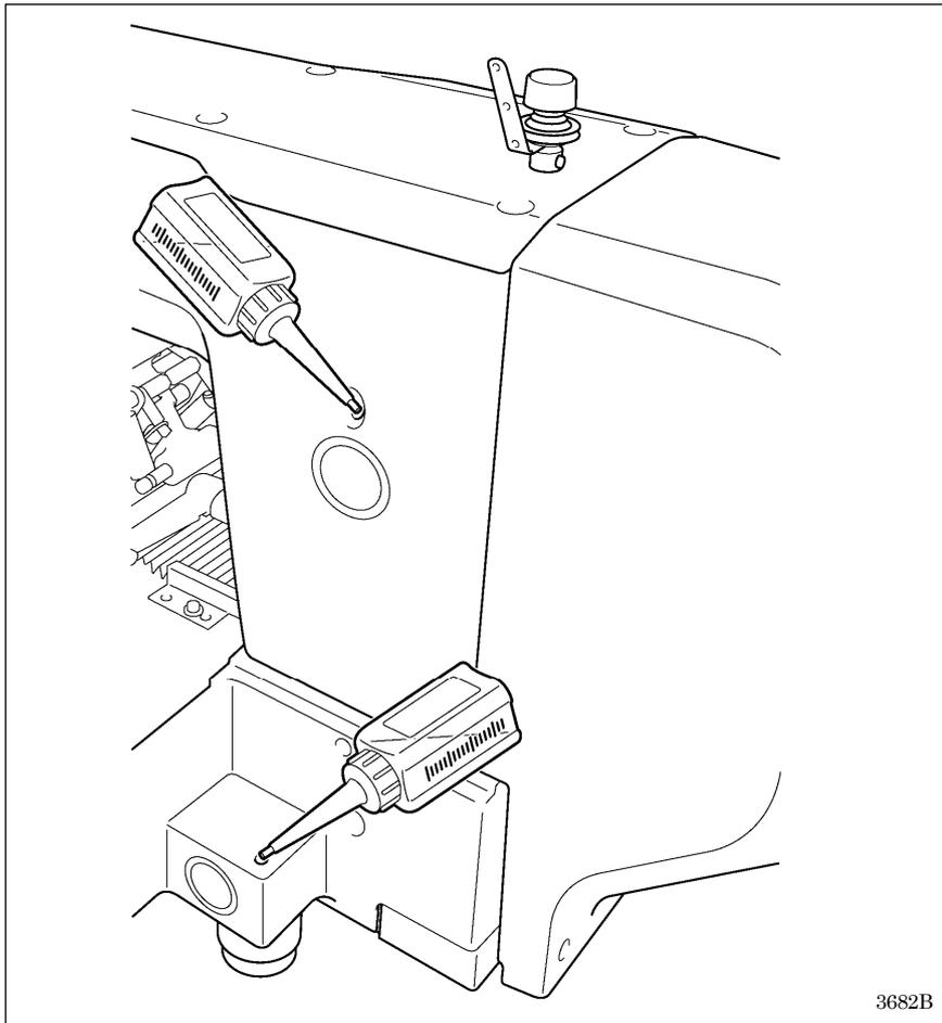
1. Fill the arm-side oil tank with oil.
