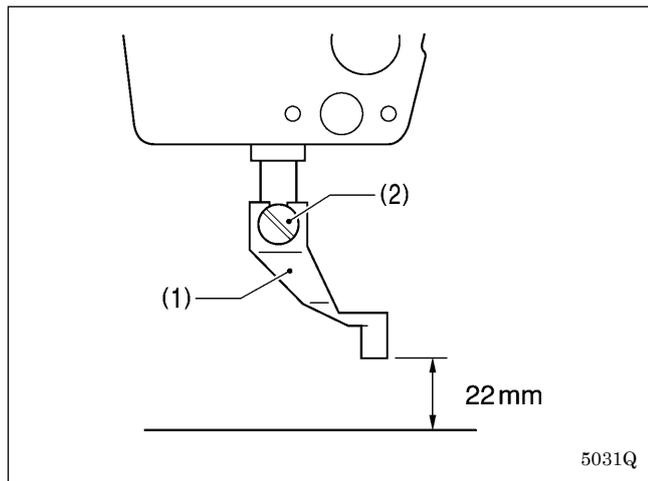
Install the intermittent presser foot (1) with the screw (2) so that the distance from the bottom of the presser foot to the top of the needle plate is 22 mm when the sewing machine is stopped and the intermittent presser foot (1) is raised.
