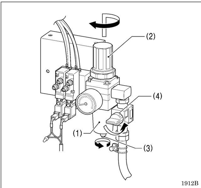
Lift up the handle (2) of the regulator (1) and then turn it to adjust the air pressure to 0.5 MPa.
