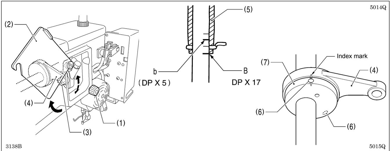
1. Loosen the screw (1), and then open the cover (2).
