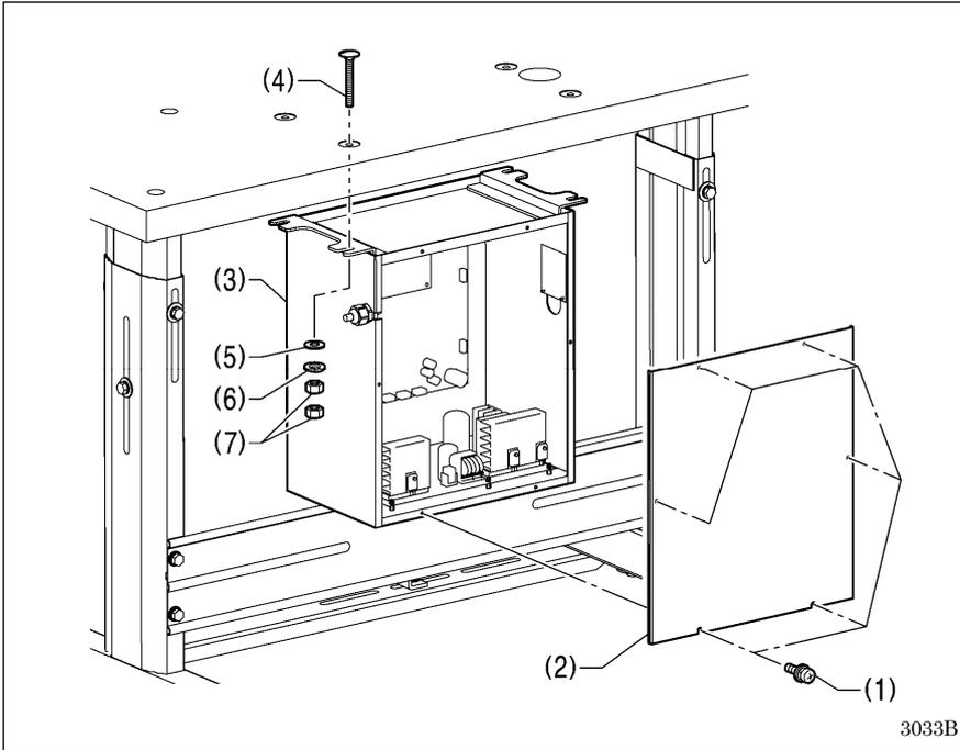
Remove the six screws (1), and then remove the control box cover (2).
