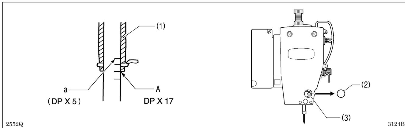
Turn the pulley in the direction of the arrow to move the needle bar to the lowest position. Then remove the rubber plug (2), loosen the screw (3) and then move the needle bar up or down to adjust so that the second reference line from the bottom of the needle bar (reference line A) is aligned with the lower edge of the needle bar bush (1).
