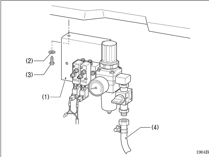
Install underneath the work table.
