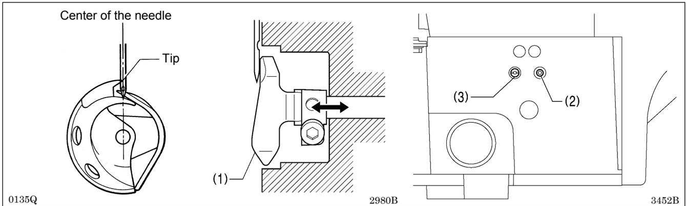
Turn the pulley in the direction of the arrow to align the tip of the rotary hook with the center of the needle, and then loosen the set screw (2) and adjust by moving the eccentric shaft (3) to adjust so that the driver (1) is touching the needle. The set screw (2) and the eccentric shaft (3) are on the right side of the bed at the rear.
