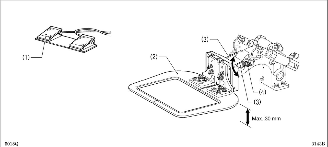
1. Turn on the air, and then depress the work clamp switch (1) to raise the work clamp (2).
