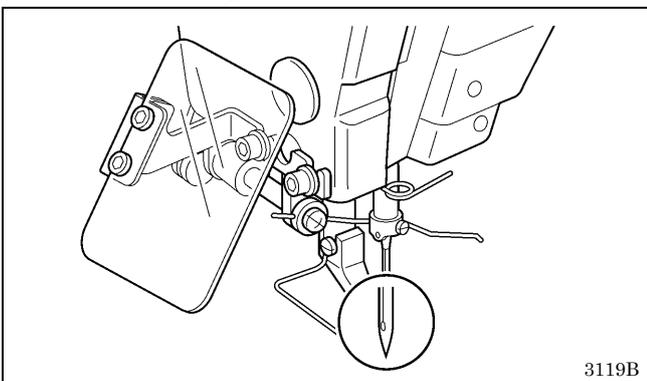
Always check that the tip of the needle is not broken and also that the needle is not bent before starting sewing.
