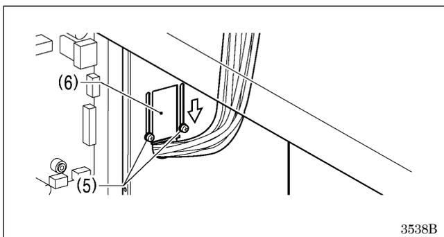
5. Close the cord presser plate (6) in the direction of the white arrow, and secure it by tightening the two screws (5).
