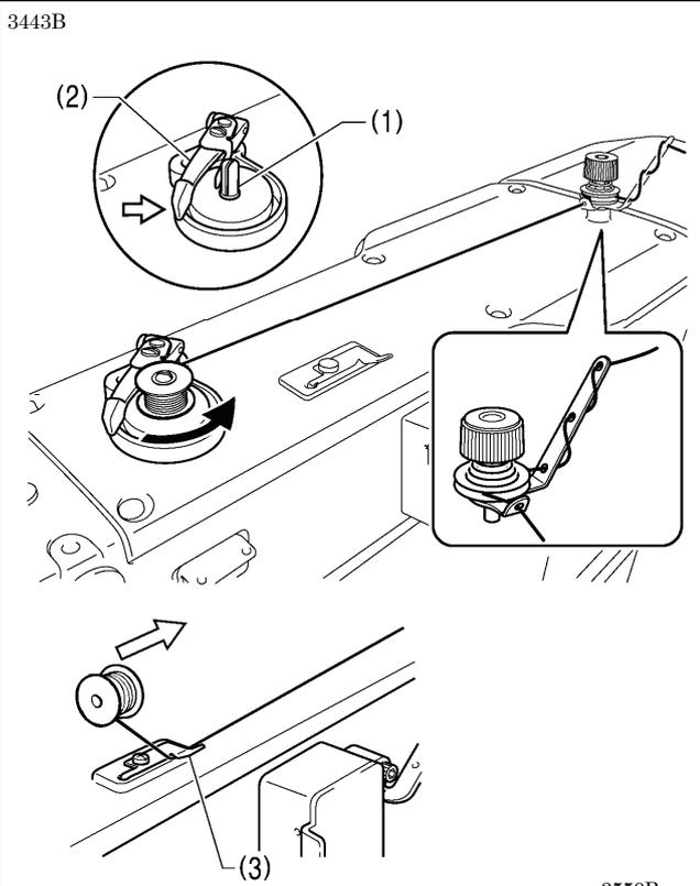
1. Place the bobbin onto the bobbin winder shaft (1).
