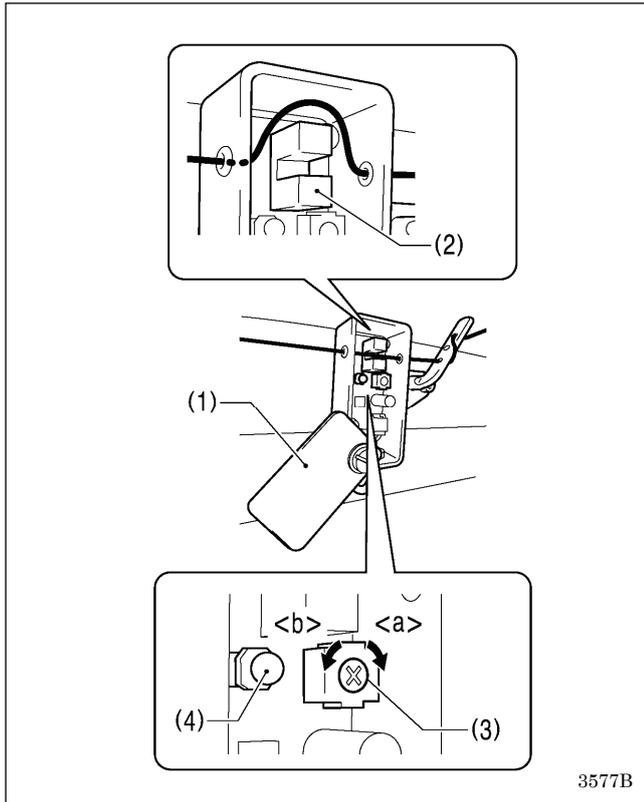
1. Open the cover (1) and remove the upper thread from the photo sensor (2).
