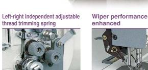
Wiper mechanism performance has been increased by approximately 60% (in-house comparison). Stable
