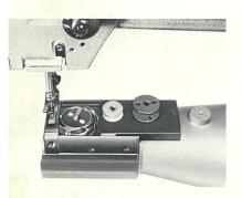
Winding volume of LCW large bobbin is more 2 times than conventional DB types. Thus, you can save a time for exchange lower thread.
