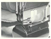
Tape binding of 2 folds, 3 folds, and 4 folds can be done by fitting of various kinds of binders.
