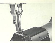
LCW-6F Upper feed with spring return presser foot, lower feed. Suitable for sewing of medium heavy weight materials, such as leather, man-made leather, vinvl. Especially, suitable for sewing of tubular products, such as leather gloves, shoes, bags, hand-bags, etc.
