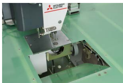
The bobbin can be replaced from the top
