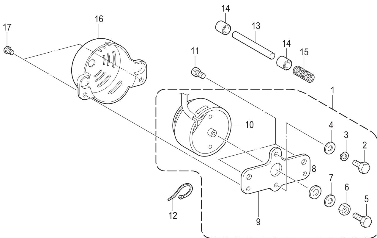
L2. 糸ゆるめ関係 (糸ゆるめソレノイド) / Tension release mechanism (Tension release solenoid)
