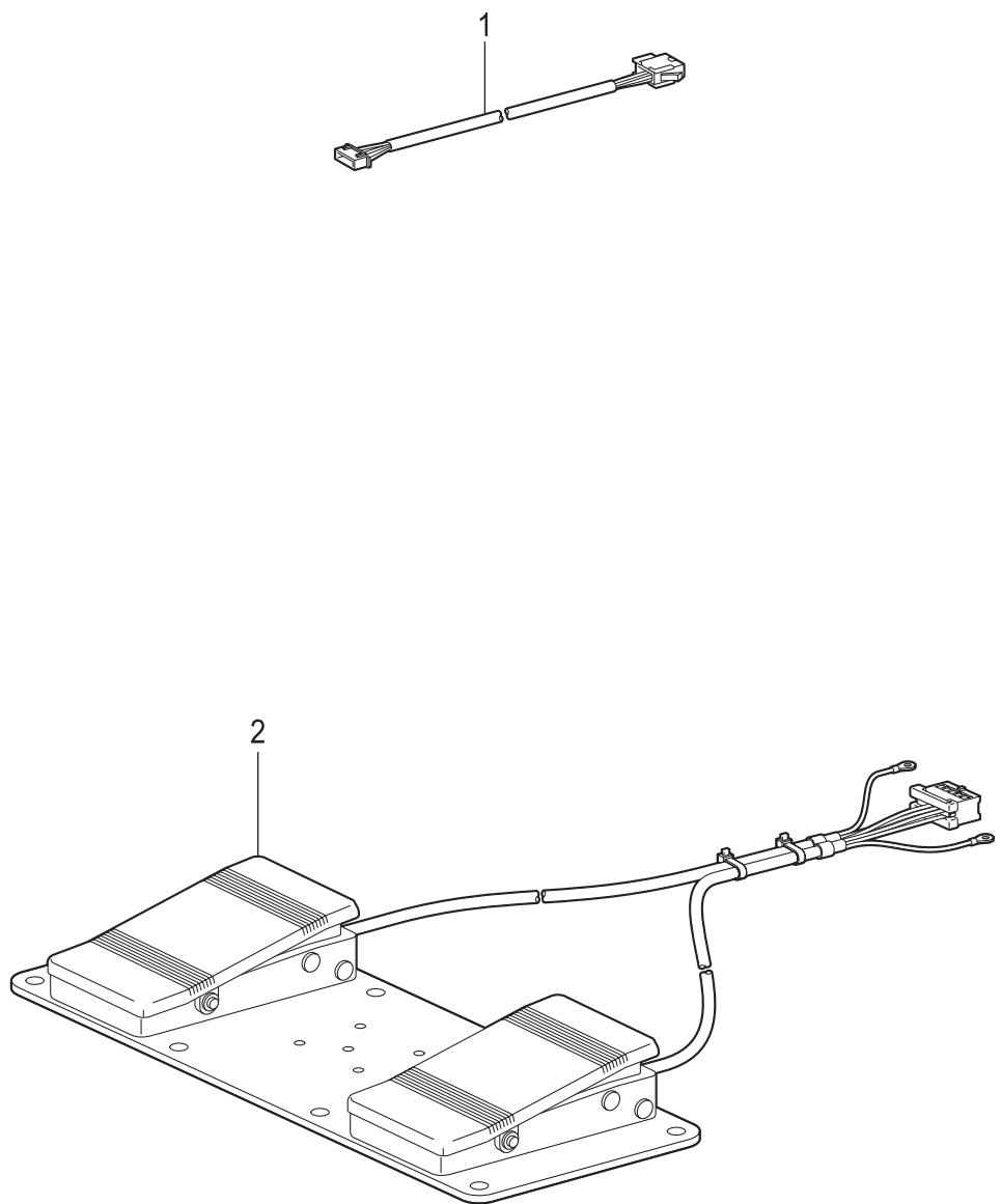
R. 踏板関係 / Foot switch pedal mechanism
