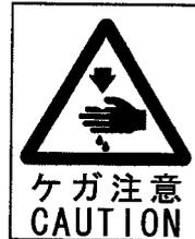
This label is affixed on the safeguards. Considering the operation, it is not affixed on the finger guard and eye guard. Be sure to operate with the finger guard and eye guard in position.
