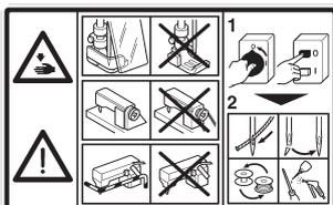
This label indicates that removal of the safeguards and works except for sewing performance while the power supply switch is on are prohibited. (For details, see the next page.)
