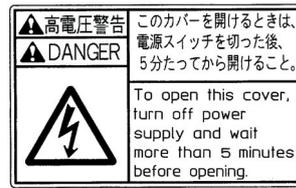
High-voltage applies in the control box. This label indicates that electric shock may be caused.
