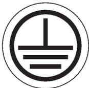
This mark indicates the caution which, if not grounded, the machine or device could malfunction and could result in personal injury.
