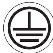
If not connected earth line, static electricity may be generated and inflict injury on person. In addition, the malfunction of electric system may cause injury to person.
