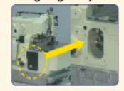
The feed dog tilt is easy to tilt up or down from outside of the machine depending on the sewing conditions.
