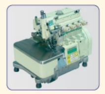
Seam width from 5mm to 8mm is convertible by simple replacement of stitch plate and presser foot tongue, without any adjustment.
