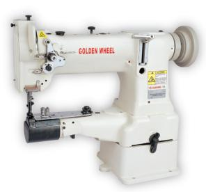
Single Needle, Unison Feed, Cylinder-Bed Sewing Machine. (Standard hook) (Horizontal movement of bottom feed, for binding stitching)
