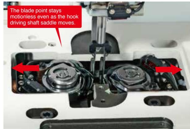
Image of adjusting the hook driving shaft saddle
