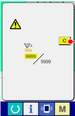
When the count-up condition is reached during sewing work, the count-up screen is displayed and the buzzer beeps. Press CLEAR button **C** **A** to reset the counter and the screen returns to the sewing screen. Then the counter starts counting again.
