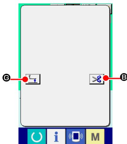
1. When the presser is raised and the operation is stopped on the way because of the trouble of forgetting to enter the bobbin case or the like, press
