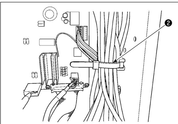
2) Secure the cable to be put into the POWER BOX with an internal cable clip ❷ .
