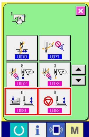
2-step stroke function can be used by changing setting of memory switches **U081** and **U082**.
