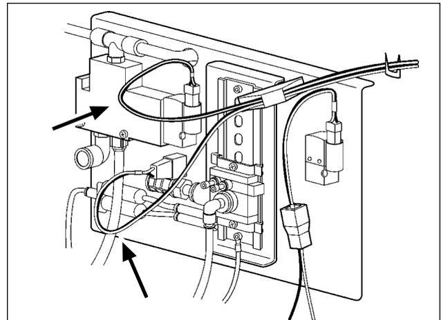
**If a cable has a slack, fix the cable on the table by means of a stapler supplied with the unit.**
