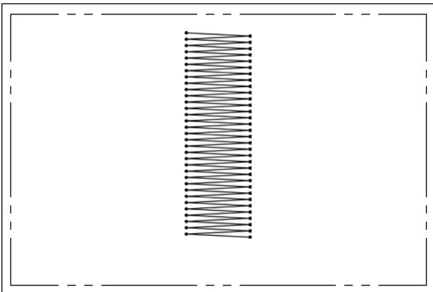
Grease film on the feed gear is likely to run out when using the machine for sewing such a sewing shape that has continuous reverse-feed stitching as shown in the figure at the left. To keep the grease film on the feed gear, carry out the following two steps of procedure.
