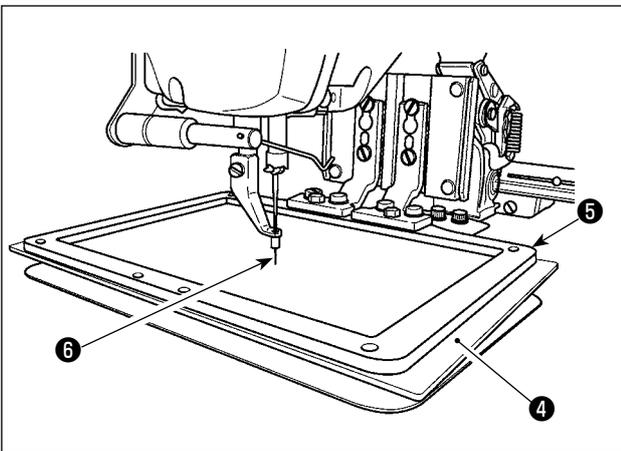
If plastic work clamp ④ is set on feeding frame ⑤ with the work clamp remained at the factory-adjusted height at the time of delivery, needle tip ⑥ can interfere with plastic work clamp ④ . To prevent the interference, adjust to decrease the work clamp height or set plastic work clamp ④ with feeding frame ⑤ held lowered by hand.
