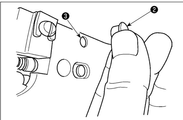
When thread is caught at top end ① of the thread clamp, thread clamp becomes incomplete and sewing trouble at the sewing start will be caused. Thread waste and lint are likely to accumulate in the sections which are shown in the circles. The sections should therefore be periodically cleaned by removing the throat plate and by blowing air through hole ③ by removing rubber plug ②.
