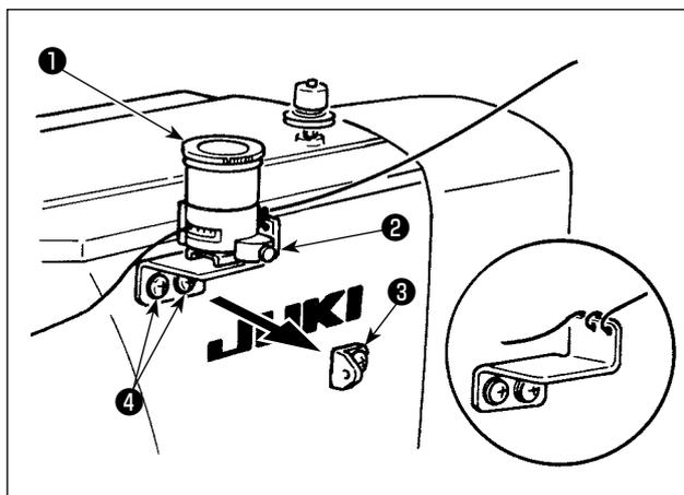
Remove take up thread guide No. 1 ③ and secure silicon oil tank base ②.
