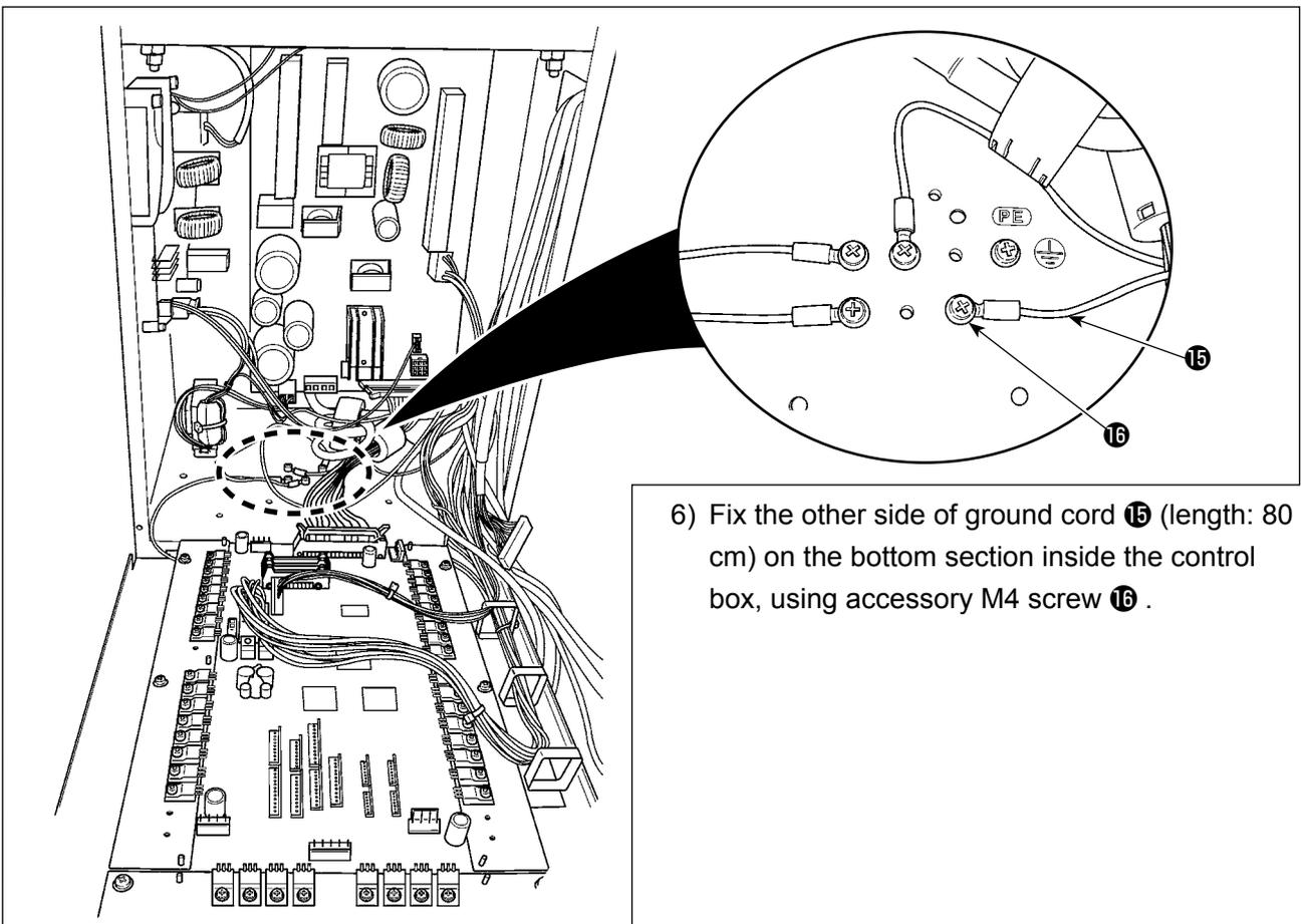
6) Fix the other side of ground cord 15 (length: 80 cm) on the bottom section inside the control box, using accessory M4 screw 16 .
