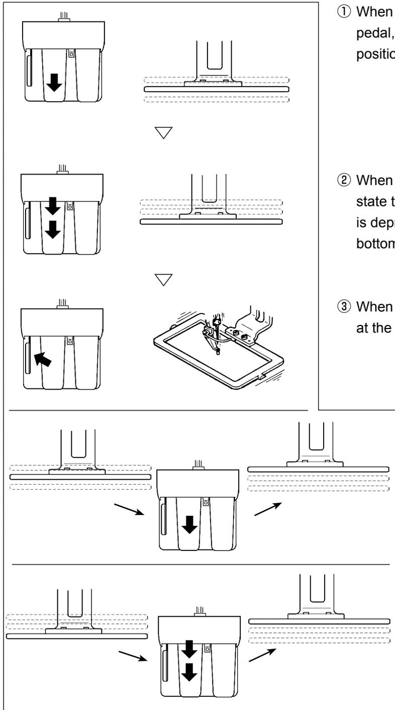
① When depressing 1st step of the intermediate pedal, the presser stops at the intermediate position.
