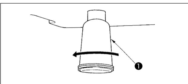
When polyethylene oiler ① becomes filled with oil, remove polyethylene oiler ① and drain the oil.
