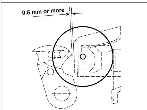
After the origin retrieval, press the SET READY key on the IP panel to verify that a clearance of 0.5 mm or more is provided between the top end of moving knife and the top end of needle thread clamp. If a clearance of 0.5 mm or more cannot be secured, adjust the position of moving knife within  $18.5 \pm 0.5$  mm to secure the specified clearance.
