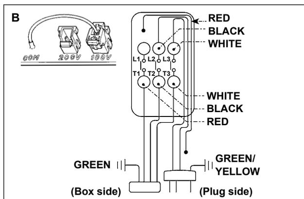
**(Caution)** Securely perform the insulation treatment to the red terminal which is not used with insulation tape or the like. (When the insulation is insufficient, there is a danger of electric shock or leakage current.)
