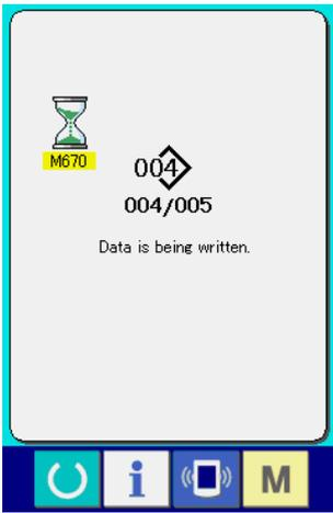
Data No. during communication, total number of writing data and number of data that have ended the data communication are displayed in the during communication screen.
