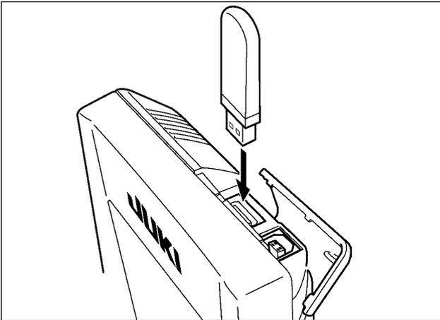
Slide the top cover and insert the USB device into the USB port. Then, copy data to be used from the USB device onto the main body.
