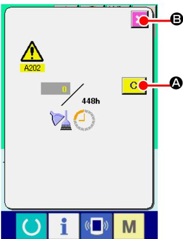
When the designated inspection time is reached, the warning screen is displayed.
