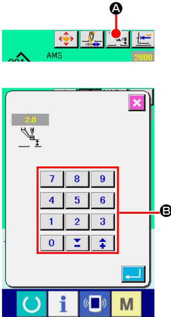
Press INTERMEDIATE PRESSER SETTING button **A** and adjust with TEN keys **B** so that the clearance between the bottom end of intermediate presser and the cloth is 0.5 mm (thickness of thread used).
