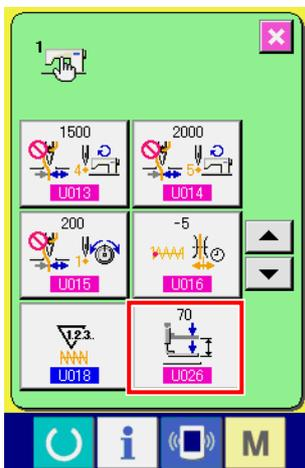
2-step stroke position used in the user's pattern can be set with memory switch **U026**.
