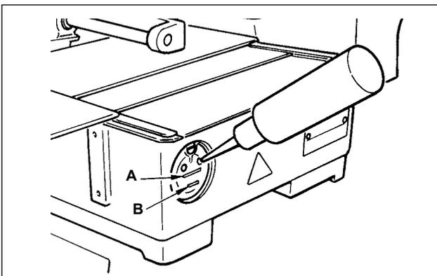
Check that the place between lower line **B** and upper line **A** is filled with oil. Fill there with oil using the oiler supplied with the machine as accessories when oil is short.
