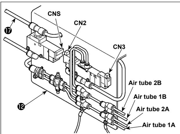
8) Install air tubes coming from the machine head to the joint of solenoid valve installing plate A asm. ⑫ as shown in the figure. Install cords (CN2, CN3, CNS) coming from the control box to the solenoid valve.
