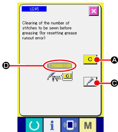
1. Error code E220 or E221 is displayed again unless NUMBER OF STITCHES **D** is changed to "0" after replenishing the designated places with grease. When E221 is displayed, the sewing machine fails to operate. So, be careful.
