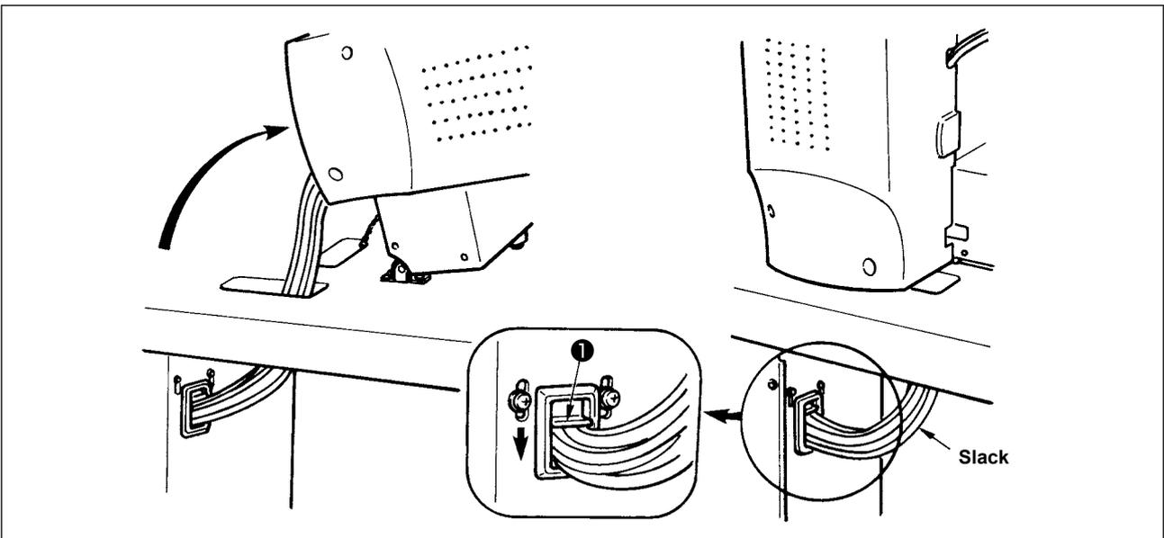
1) Fix the cords with cords setting plate ❶ in the state that the cords are slack to such an extent that stress is not applied to the cords even when the machine head is tilted as shown in the figure.
