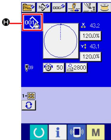
When X/Y enlargement/reduction ratio, thread tension, intermediate presser, adding/deleting of thread tension command, or adding/deleting of increase/decrease value of intermediate presser of users' pattern or media pattern is performed, the pattern kind section becomes change display **H**.
