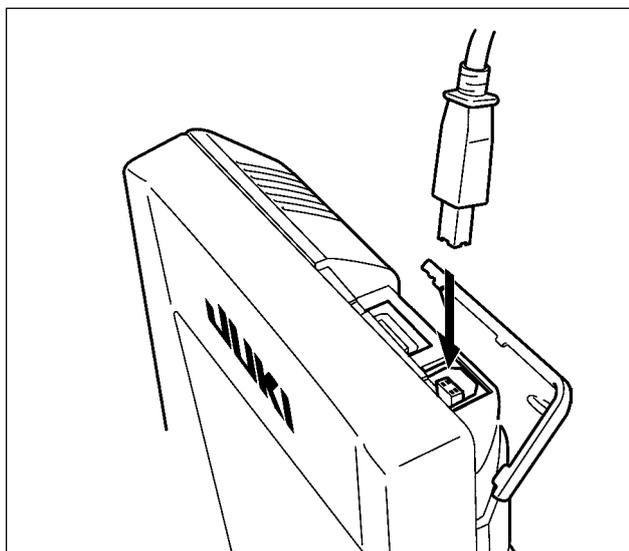
Data can be sent/received to/from a personal computer or the like, by means of a USB cable.
