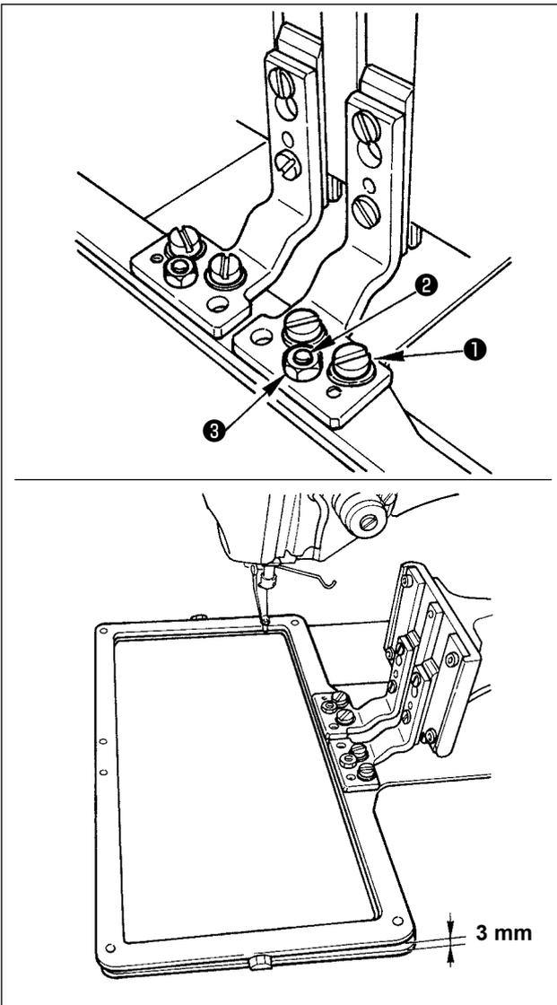
If the feeding frame is in parallel to the throat plate, the pressure of the front side of the feeding frame is likely to drop. Consequently, be sure to adjust the inclination of the feeding frame so that the front side of the feeding frame is slightly lower than its rear side.
