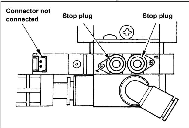
6) Install the retaining plugs supplied as accessories with the machine to solenoid valve asm. ⑧.
