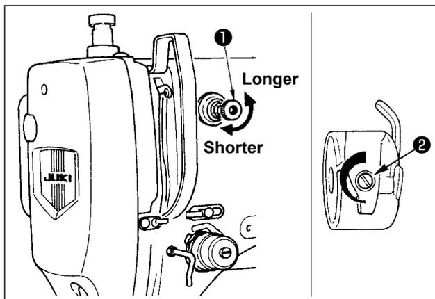
If thread tension controller No. 1 ① is turned clockwise, the length of remaining thread on the needle after thread trimming will be shorter. If it is turned counterclockwise, the length will be longer. Shorten the length to an extent that the thread is not slipped off.
