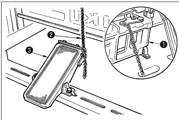
Connect the machine ① and manual pedal ③ with chain ②.
