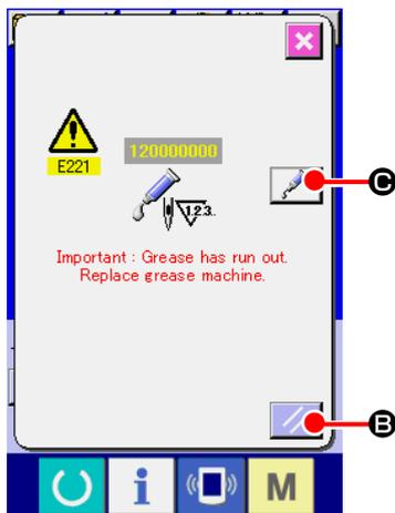
When error "E221 Grease-up error" is displayed, be sure to replenish the designated places below with grease. Then call the memory switch U245, press CLEAR button
