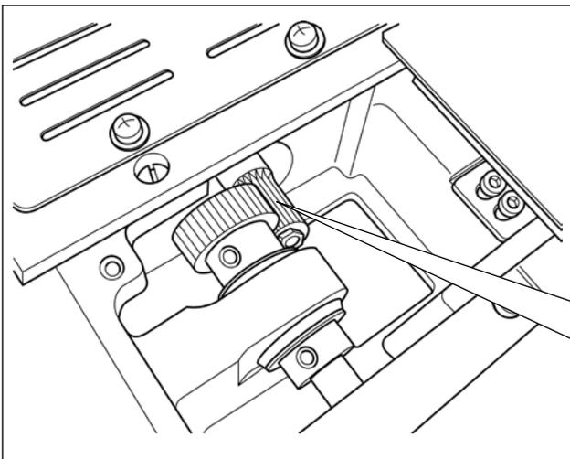
For the sewing shape as shown in the figure, only a part of the gear is continuously used. Apply the grease to the mesh of the gear which is used for sewing.
