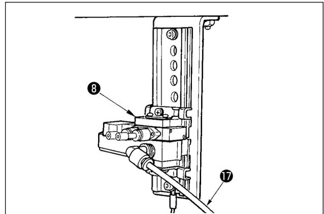
7) Connect air tube ⑰ of solenoid valve installing plate A asm. ⑫ solenoid valve asm. ⑧.
