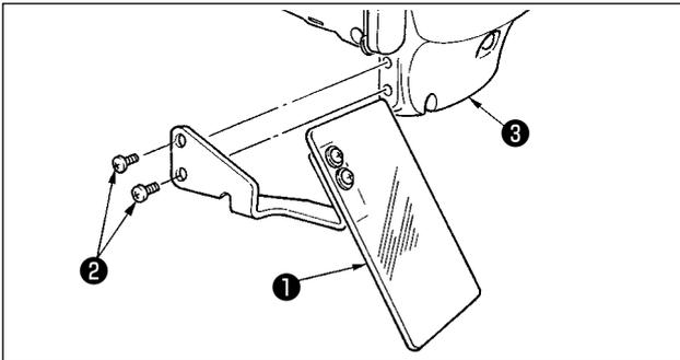
Use eye protection cover ① after securely attaching it on face plate cover ③ with screw ②.
