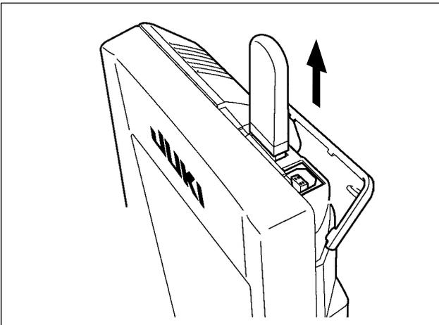
Remove the USB device. Put the cover back in place.
