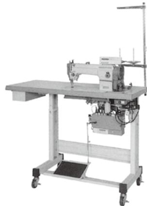
Single-needle lockstitch: Vertical feed (cylindrical high-long arm)
