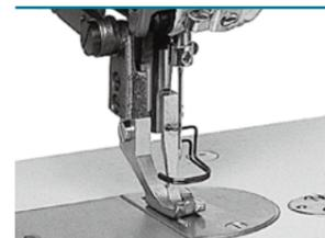
The vertical feed sandwiches and accurately feeds hard-to-feed materials.
