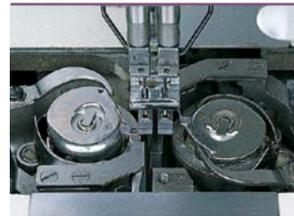
A moving knife and fixed knife that move linearly in parallel with the feed gear are used to cut thin to thick threads (#8) with a clean cut.
