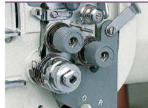
Thread tension can be adjusted for the left and right threads. Adjustments are easy to make, and stepped stitching such as stitching collars turns out beautifully.
