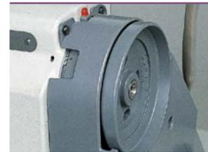
Needle stop UP and DOWN positions can be adjusted separately with a single touch. The normal state can be confirmed easily via indicator lamps.
