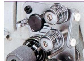
Low-wear ceramic materials are used for the thread route in the thread tension regulator, resulting in a dramatic improvement in durability.
