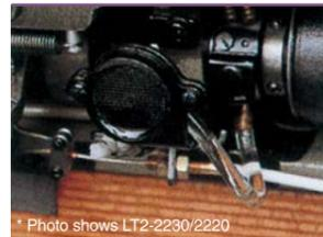
The automatic lubrication system eliminates the need for manual oiling. A pump feeds oil in the oil tank to the required sections, further improving sewing machine durability.
