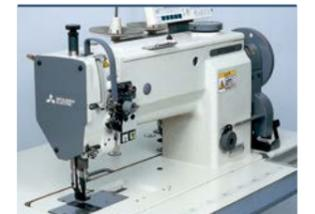
With the improved needle bar vibration mechanism, balance mechanism and upper vertical feed mechanism, machine can do up to 3,000 stitches/min even when using a double-hook. (Only LU2-4652)
