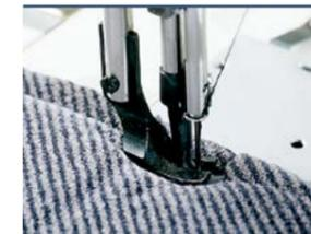
CS specifications have been added to the car seat stitching lineup. The balance stroke and feed motion have been changed and seat stitching quality has been further improved.
