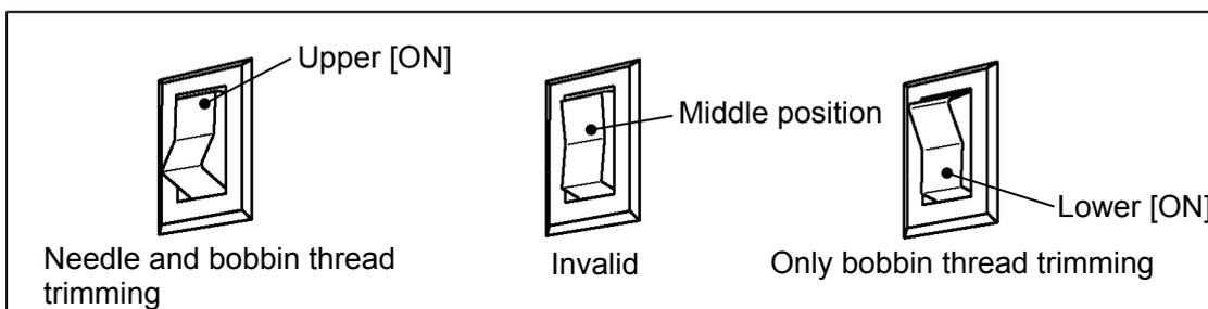
Thermal thread trimming device switch needs to operate according to below procedures.
