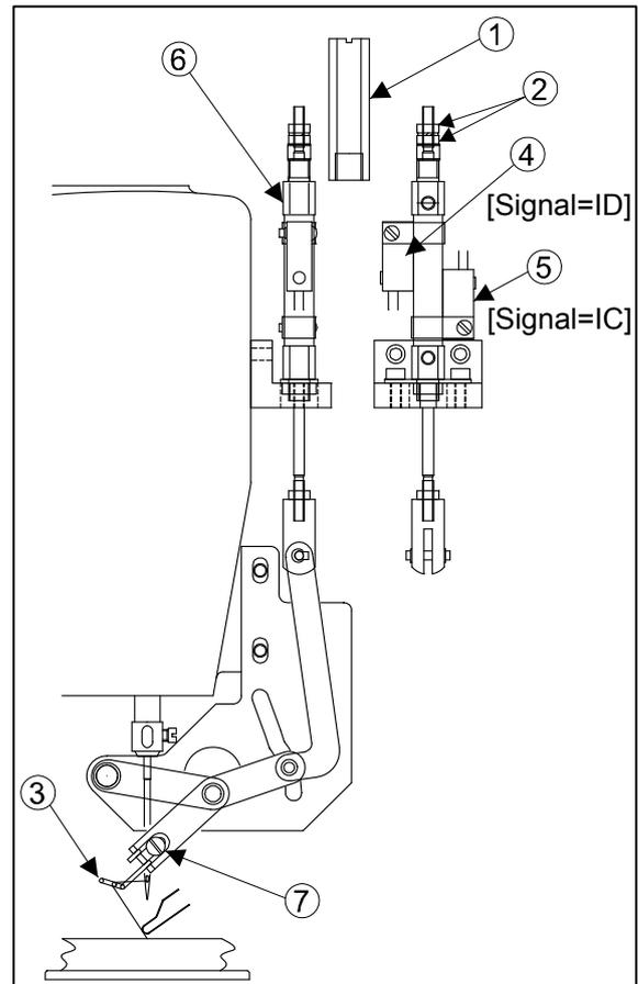
The thread wiper should move freely past under the needle. To correct the height of the thread wiper
