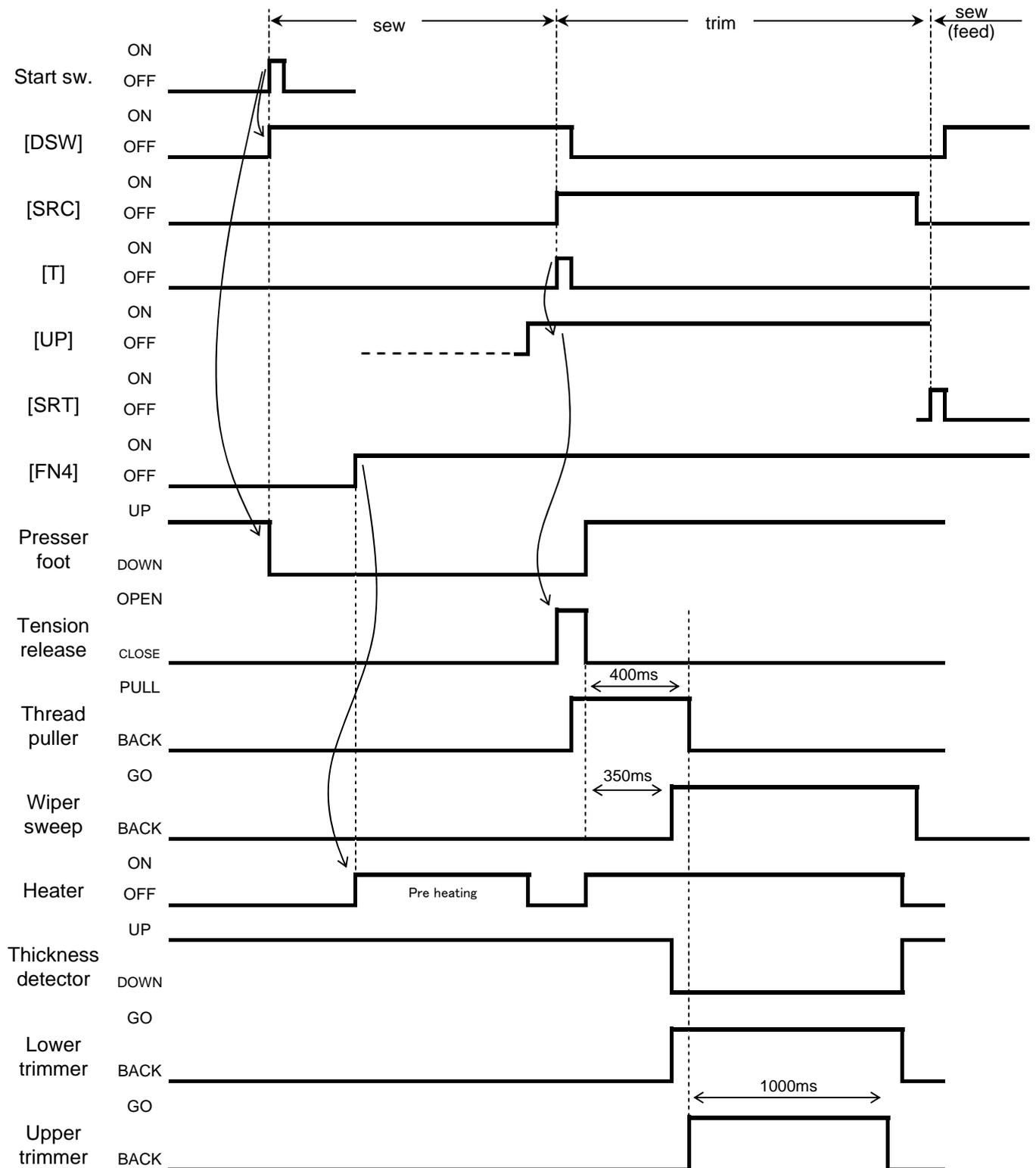
[DSW] : Sewing in progress output signal (by system)
