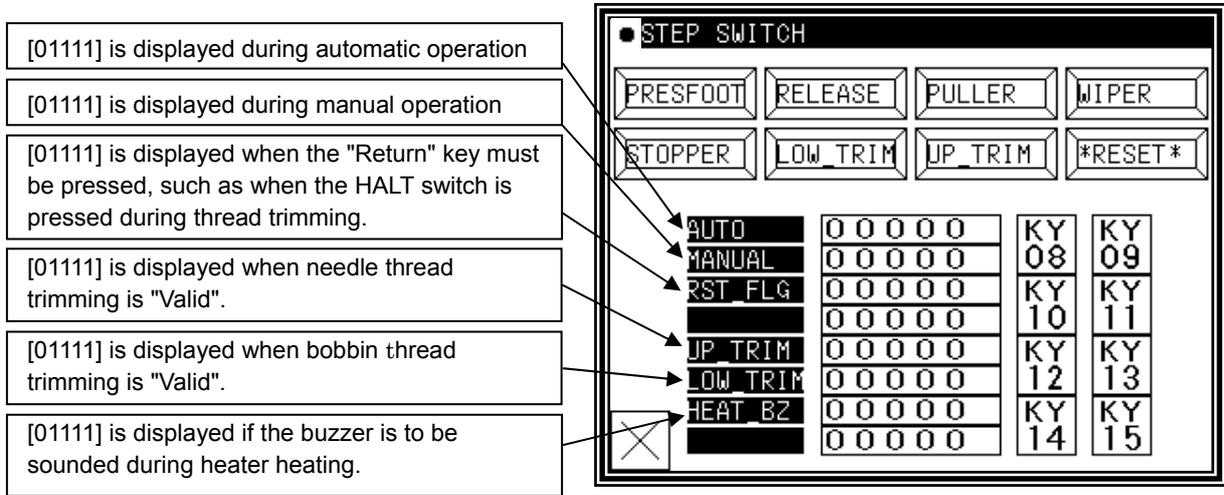
\* The state with each key pressed and highlighted is the [ON] state.
