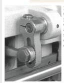
By changing the support point position of the crank rod, the alternating stroke amount can be adjusted easily.
