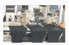
缝合压线一次完成 Stitching and pressing are completed at one time
