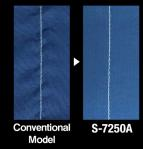
5 Short remaining thread, (3mm) doesn't require after-cutting process
