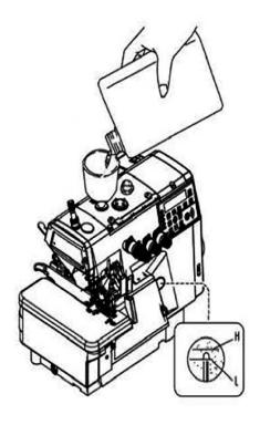
After filling the oil pan. the top of the indicator should lie between (H) and (L) lines.
